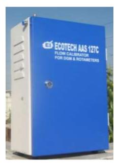
The AAS 127C an intermediate calibration checking system fitted with master DGM and stop watch along with connector and tubing which can be used for calibration of DGM either in situ of instrument or an independent unit for flow rate in field.
